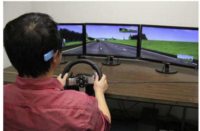
**Fig. 1.** HyperDrive driving simulator with driver wearing Google Glass.
