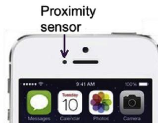
Fig. 3. Demonstration of the proximity sensor in Google Glass and iPhone.
