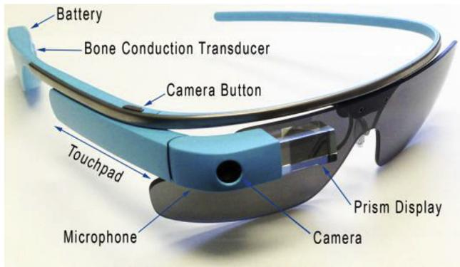
Fig. 2. Google Glass with structure labels.
